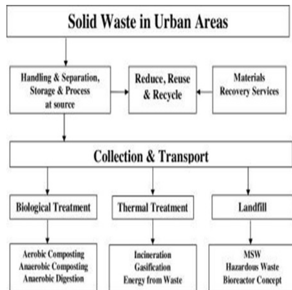
Fig:4.2.2 Flowchart representing the processes involved in solid waste management in Urban areas
