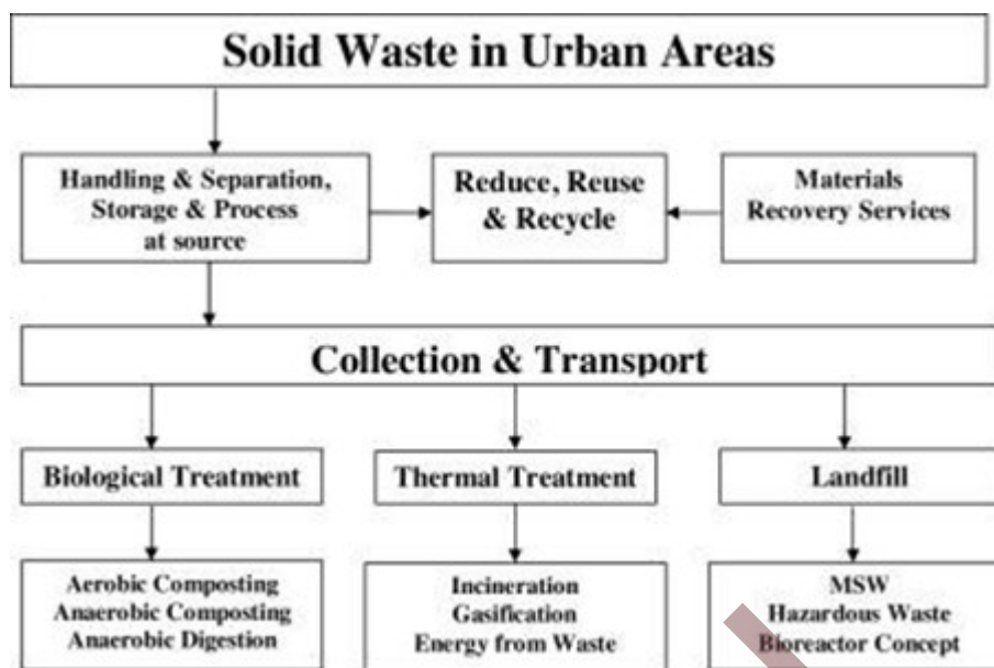
Fig 2.1.3 Flowchart representing the processes involved in solid waste management in Urban areas
