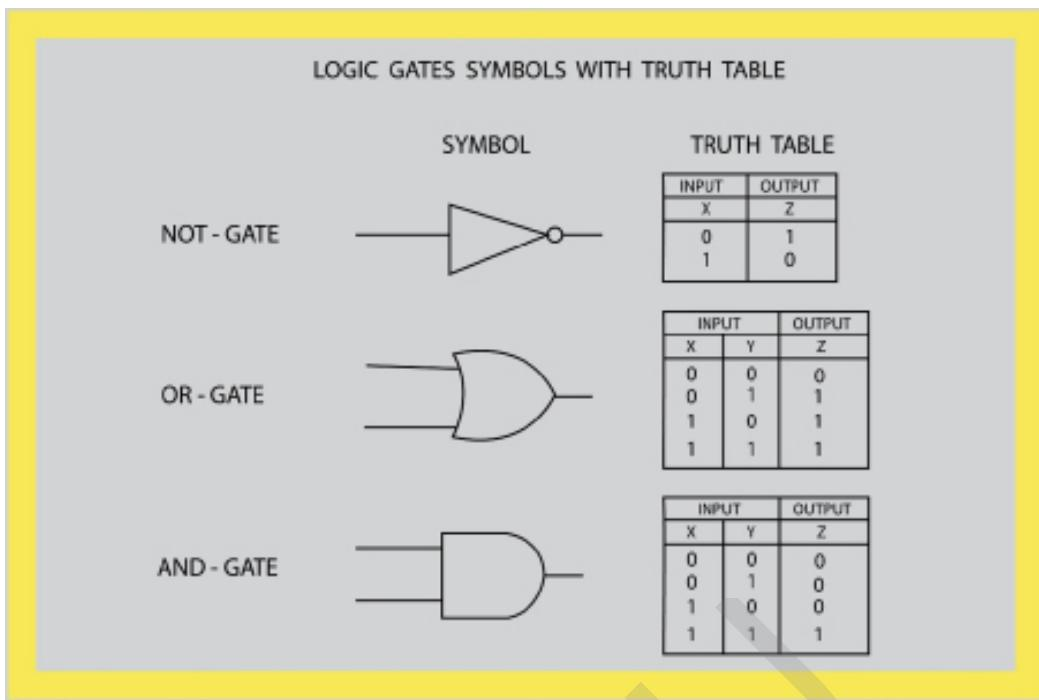
Fig. 3.2.1 Logic gates symbols with truth table
